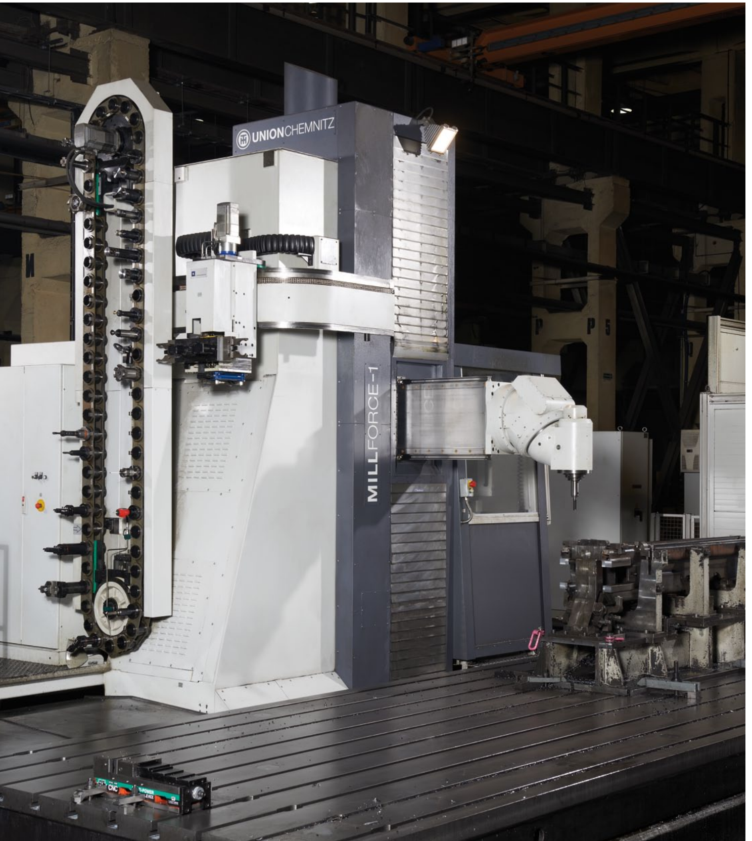
Universal travelling column mill for producing single pieces as well as small and medium batches.
