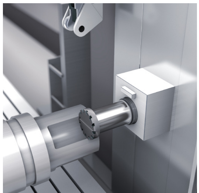
Milling a wobbler neck, parallel to Z-axis
