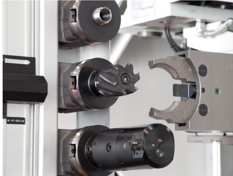
Automatic tool change from the magazine
